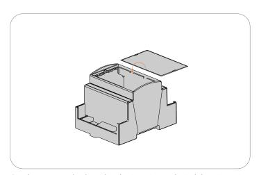
Put the top cover back on the plastic casing and mind the orientation of the label.
