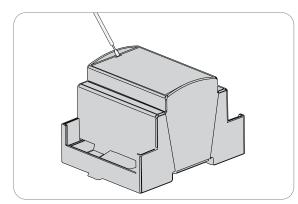
Insert the tip of a flat screwdriver (4.0 x 50 mm or similar) in the small opening on top of the driver.
