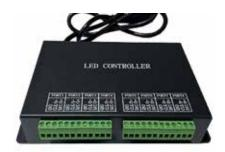
H801RC is a slave controller that transmits data based on Ethernet Protocol, data is input from mater controller or computer to NET1 and output from NET2. H801RC has eight output ports and drives maximum 8192 pixels, and can be connected to computer or master controller.
