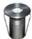
RECESSED LIGHT R38 1,6W 30D 24V 3000K IP68 INOX 316
